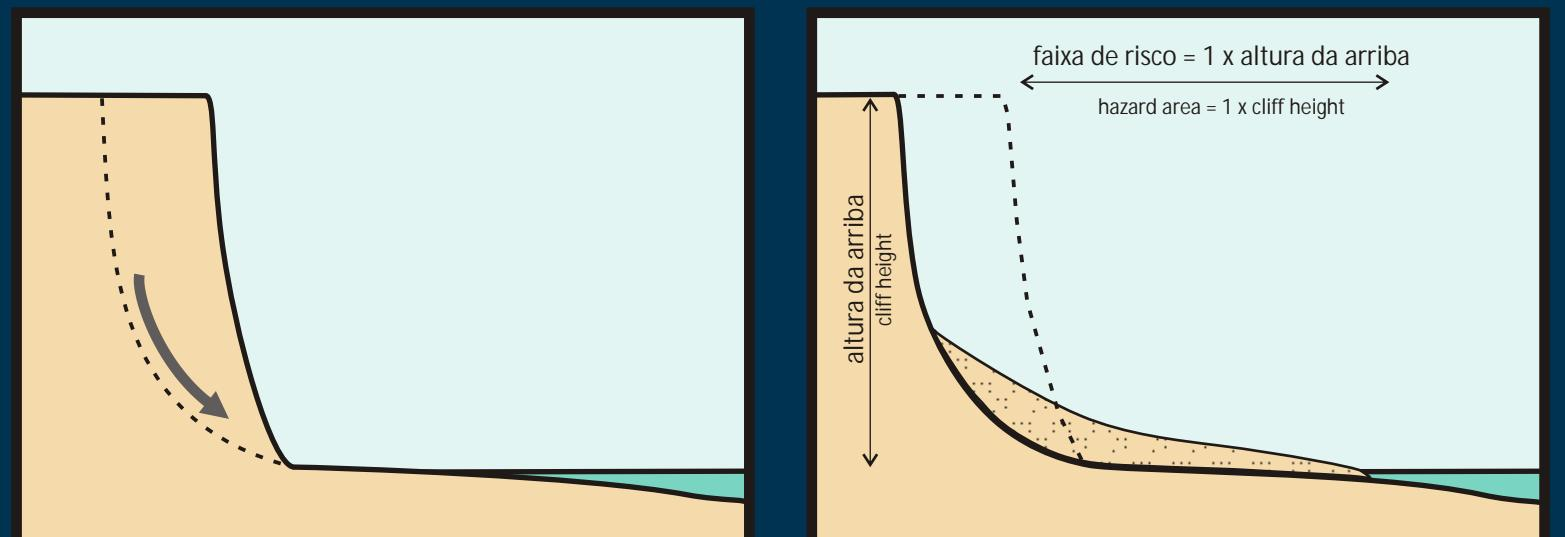
Natural cliff evolution (erosion) progresses by intermittent and discontinuous series of rockfall and cliff collapses. Cliff evolution is a potential menace for people standing on beaches accumulated at the cliff base. HAZARD AREAS correspond to areas where it is likely that effects of debris will be felt and its length equals 1 time cliff height. For your safety, keep away from cliff base and cliff edge.
